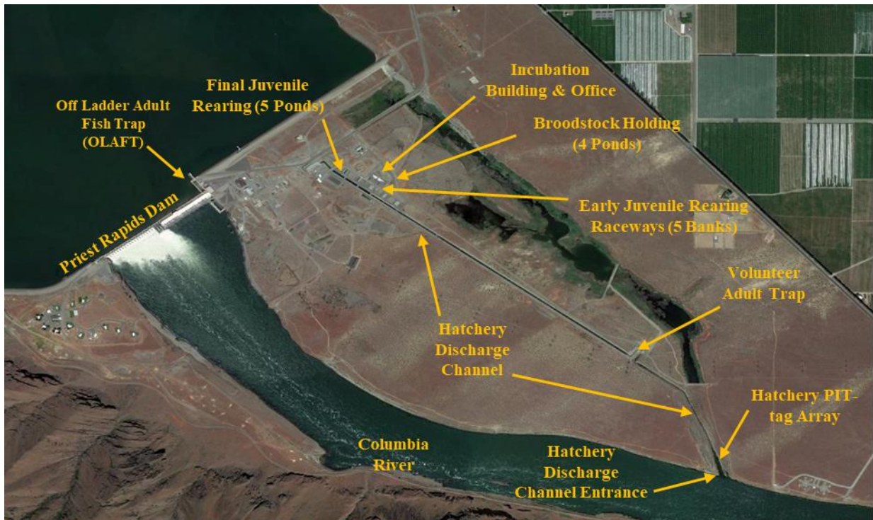
Figure 2. Priest Rapids Hatchery facility and Priest Rapids Dam Off-Ladder Adult Fish Trap.
